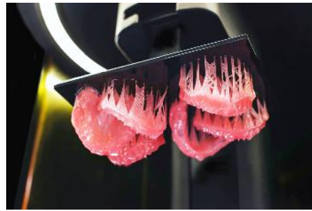
Fig. 1 – 3D printing procedure - Dentca denture base for carbon printers (1)
